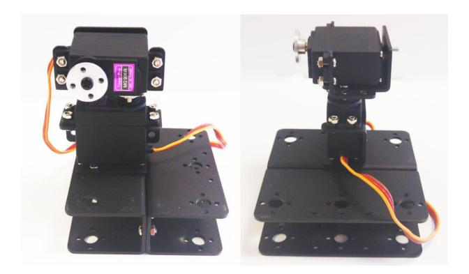
The sixth step, fix the long U-shaped on the servos and install the bearing. And fix the same long U-shaped on the long U-shaped.
