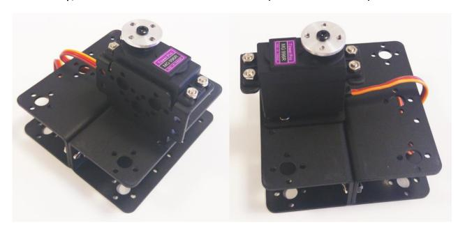
The forth step, fix a multi-bracket on the servos and insert the M3\*10 screw in the middle of the left side.
