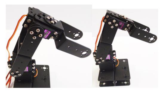
Fix the 2 Multi-bracket together (the screw is M3\*6).
